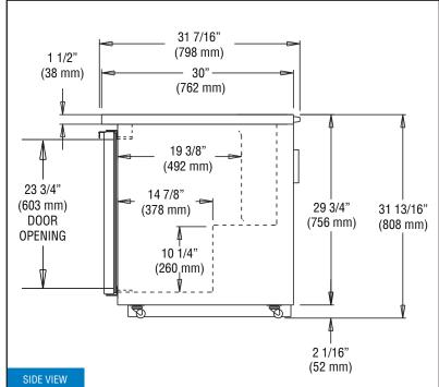
**NOTE:** For proper operation, the area under and in front of the cabinet **must** not be obstructed in any way.
